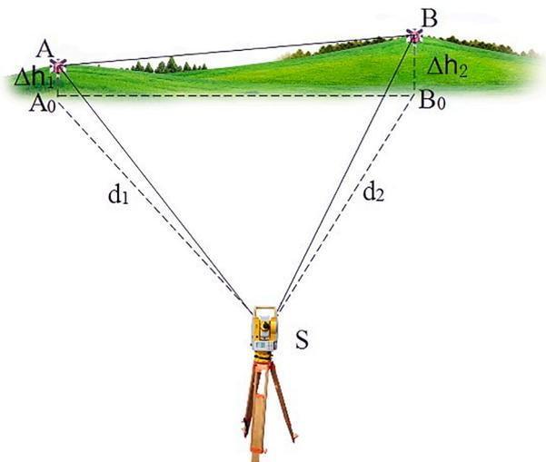
Fig. 2. Resection principle diagram. S is the installation position of the total station,  $A_0$  and  $B_0$  are the points projected onto the horizontal plane by A and B, respectively;  $\Delta h_1$  and  $\Delta h_2$  represent the elevation difference between A and  $A_0$  and the horizontal plane, respectively;  $d_1$  and  $d_2$  represent the horizontal distance from S to target points A and B, respectively.
