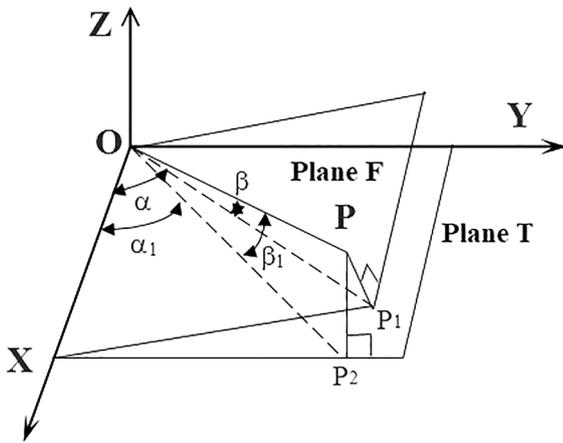
Fig. 5. Schematic diagram of angle error caused by leveling error of the instrument.
