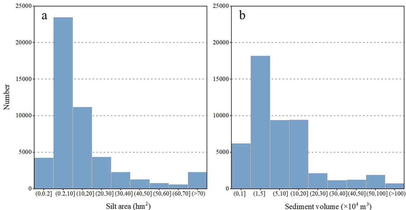
**Fig. 2** Quantitative distribution characteristics of check dams on the Chinese Loess Plateau. **a** Frequency distribution of silted area. **b** Frequency distribution of sediment volume.
