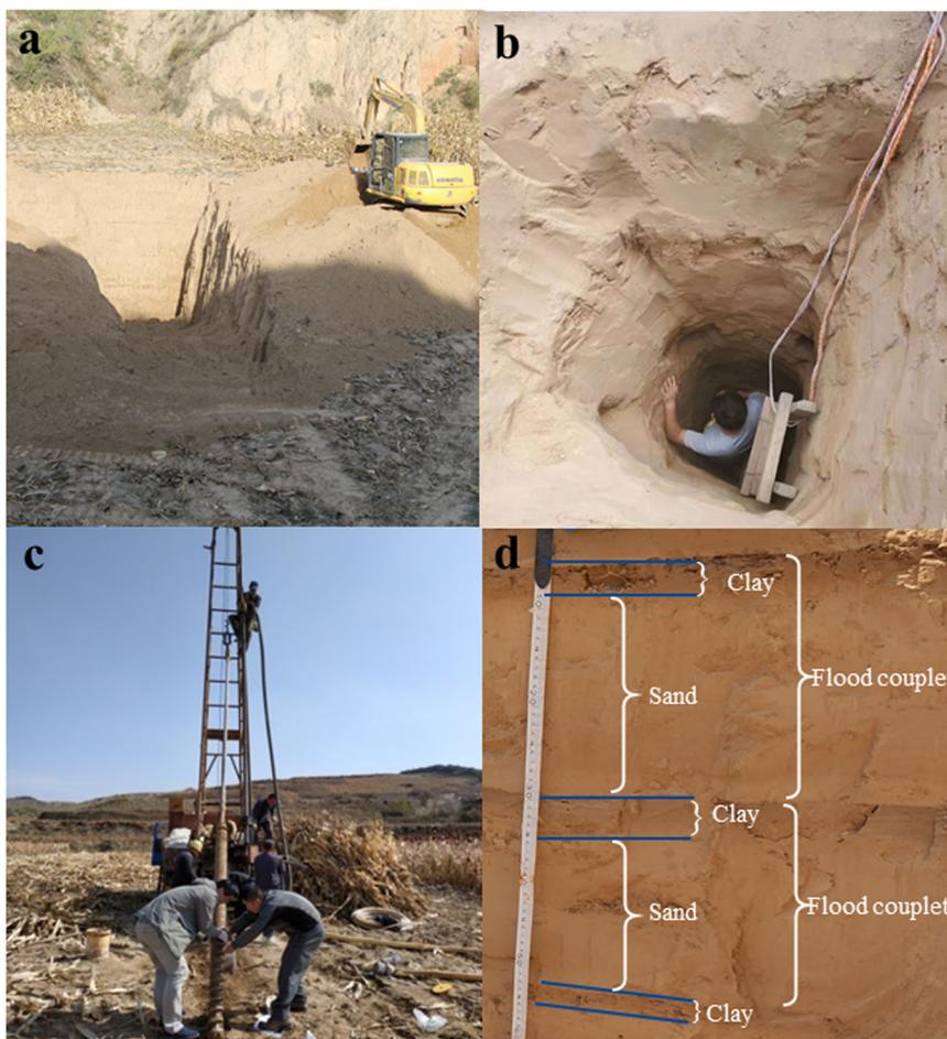
**Fig. 4** Different sediment sampling methods. **a-c** Excavator, manual well digging, and well-drilling machine. **d** Flood couplets with clay and sand layer.
