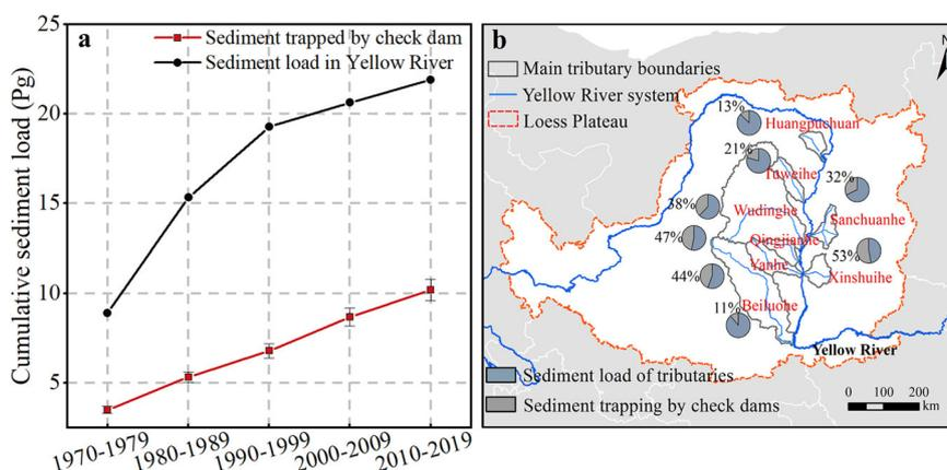
**Fig. 3** Check dams trapped sediment. **a** Sediment trapped by check dams and sediment load of the Yellow River at different historical stages. Error bars represent standard deviation. **b** Sediment retention benefits of check dams in 8 main tributaries of the Yellow River. The river sediment load data is provided by the national basic hydrological station at the outlet of each basin, without error bars.
